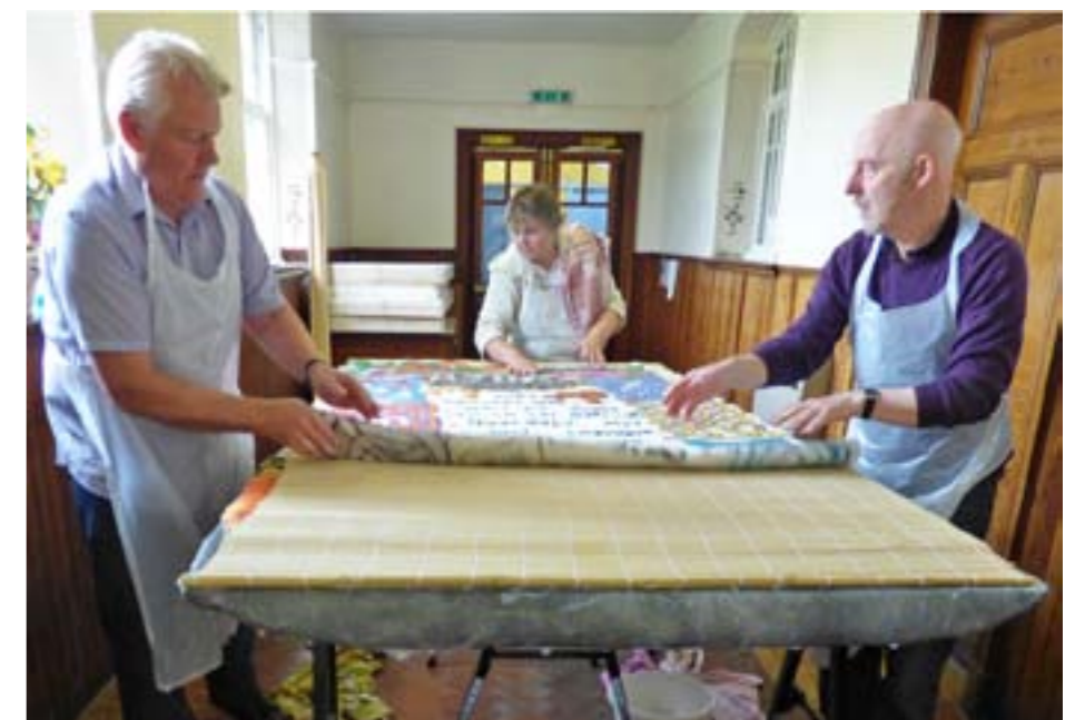
The felt had to be milled and this involves spreading the felt on bamboo mats before rolling up like a swiss roll and then rolling back and forth.
